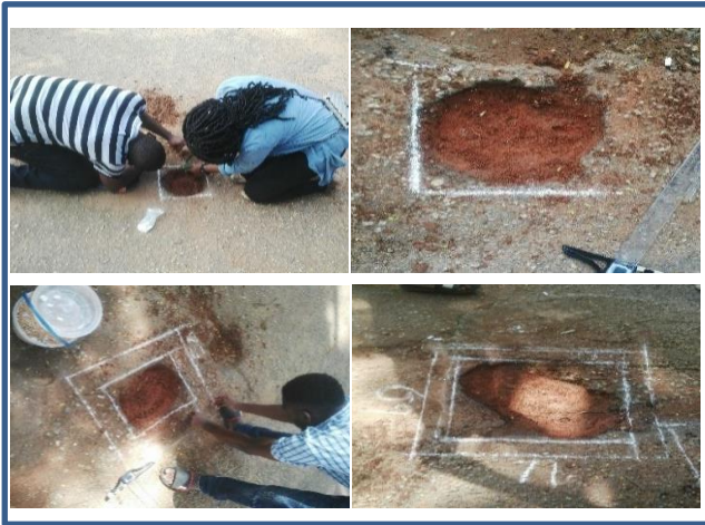
Figure 2. Pothole samples showing the marking out and manual measurement procedure.
