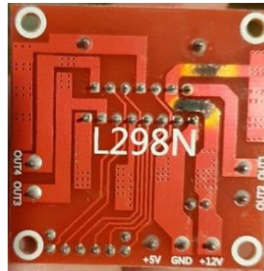
Figure 6. Burnt out L298N voltage regulator
