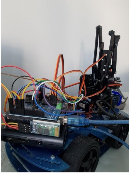
Figure 3. Arduino and Raspberry Pi 3 circuit setup
