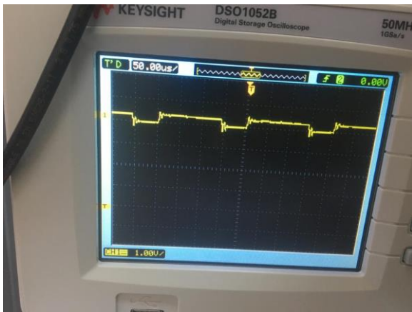
Figure 15. Output voltage waveform of two-phase interleaved DC-DC boost converter circuit with coupled inductors (inverse coupling connection).
