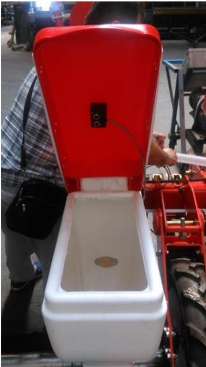
**Figure 7.** The montage of ultrasonic distance meter on seed tank
