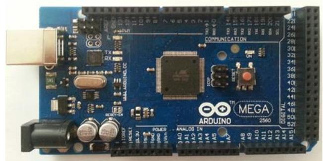
Figure 2. Arduino Mega 2560 Development Board.
