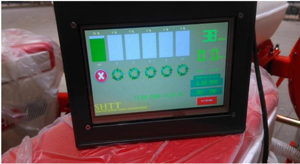
**Figure 8.** The boxed Nextion NX8048T070 TFT screen that used as graphical user interface
