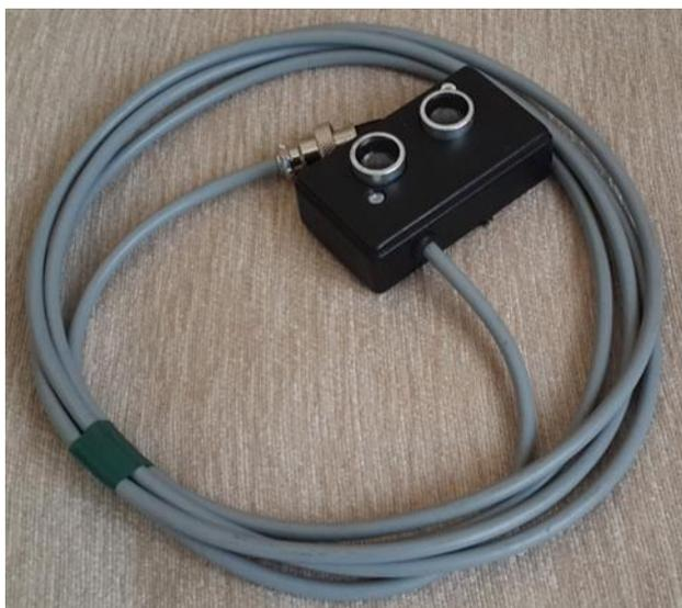
**Figure 4.** The packaged ultrasonic ranging module HC - SR04.
