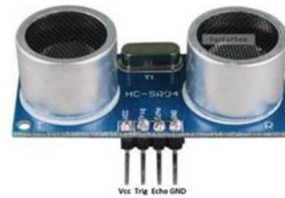
Figure 3. The tanks ultrasonic ranging module HC-SR04.
