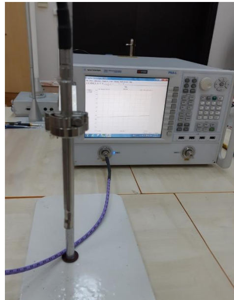
Figure 1. VNA and Coaxial Probe Measurement
