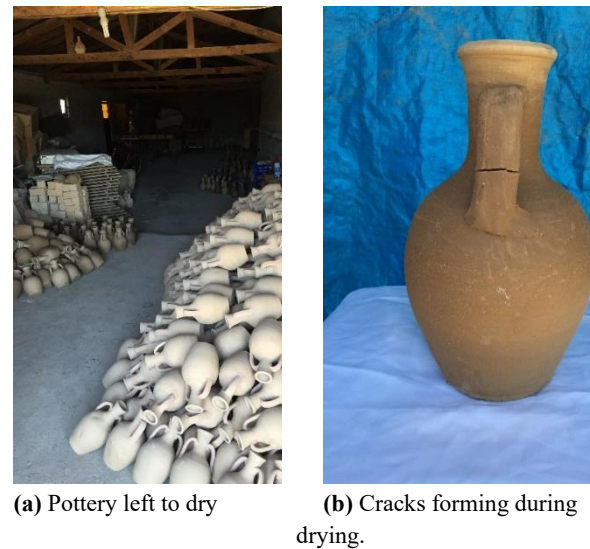
Figure 2. Drying process and defects
