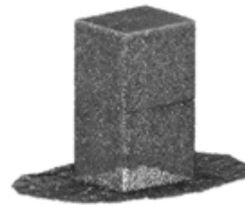
Figure 5. Sample material of known size is used to calibrate accuracy.
