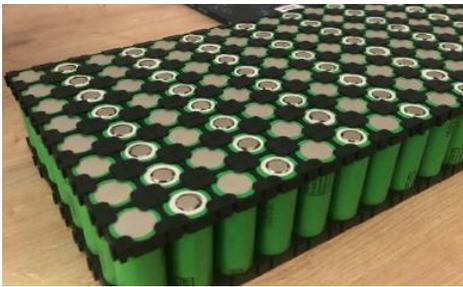
**Figure 1.** 28S8P Battery pack display
