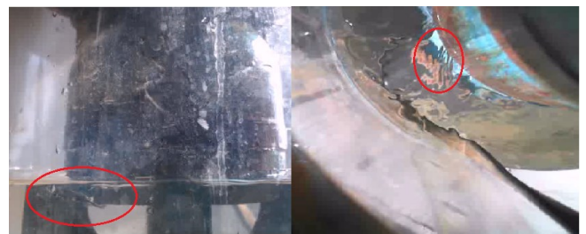
Figure 5. The images of vortex cavitation (Q=60 m 3 h -1 ;S=20 mm)
