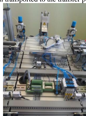
Figure 12. Fluidic Muscle Press station
