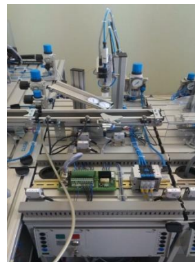
Figure 11. Pick & Place station
