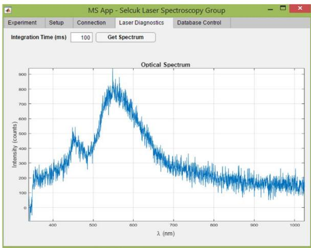
**Figure 2.** In laser diagnostic section the user can read UV-VIS spectrometer for desired integration time in ms time scale and spectra are plotting real time in the optical spectrum figure area.
