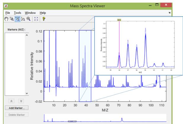
**Figure 5.** MS Viewer window opens when the user clicks MS Viewer button seen in Fig. 3. The user can select desired peaks to build a marker list into the left-hand side section.
