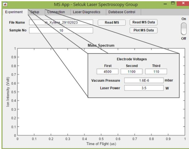
**Figure 1.** GUI of the MS spectrometry program and subpages; Experiment, Setup, Connection, Laser Diagnostics, Database Control. Setup section presented as an inset.
