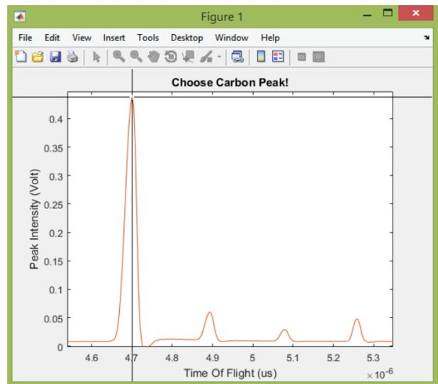
**Figure 4.** Reference peak selection on the read MS spectra to perform time of flight to mass spectrum transformation.
